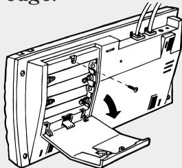
Insert 4xAAA alkaline batteries (not included) as shown in the compartment, then replace the cover.
