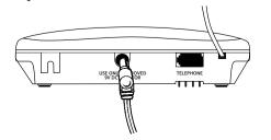
Plug the adaptor into a mains power socket
